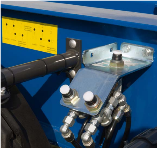
Protected mounting: The control unit for the rear extension and locking mechanism.
