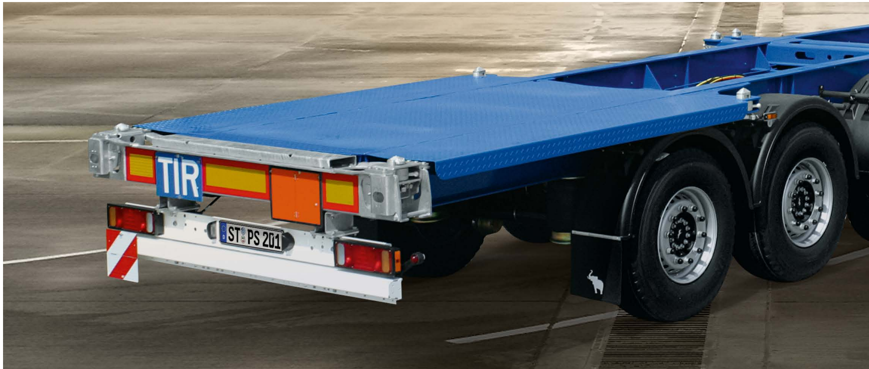
Greater flexibility when loading and unloading: Stacker-assessable rear platform.
