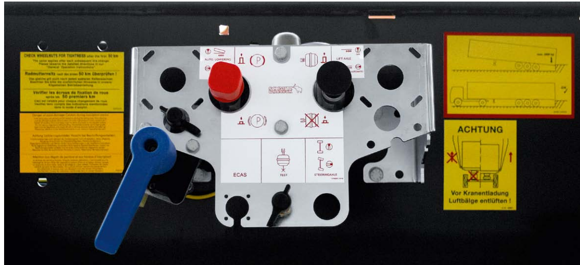
Control unit for the parking brake, axle lift and pneumatic suspension.
