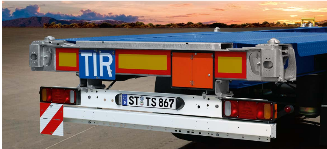
All of the signage options: Hazardous goods sign / TIR sign for transport under customs seal / Reflective night parking sign.
