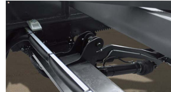
When transporting 45' containers the tail lift can also be extended via a rack and pinion gear to create an underride guard.
