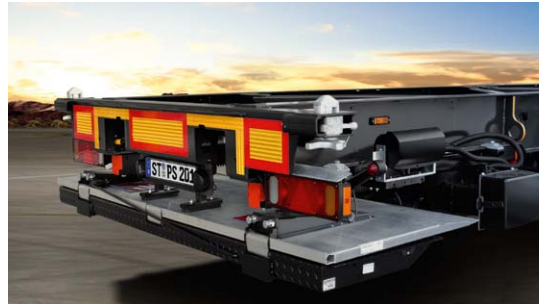
For the S.CF GS 40'/45' LIGHT: The tail lift enables loading and unloading without a ramp.
