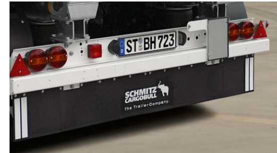
Vehicle-width spray guard on the rear.
