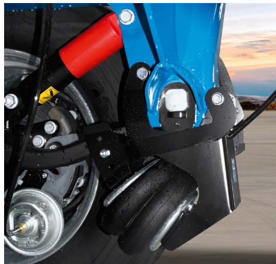
Automatic axle lift on the first axle.
