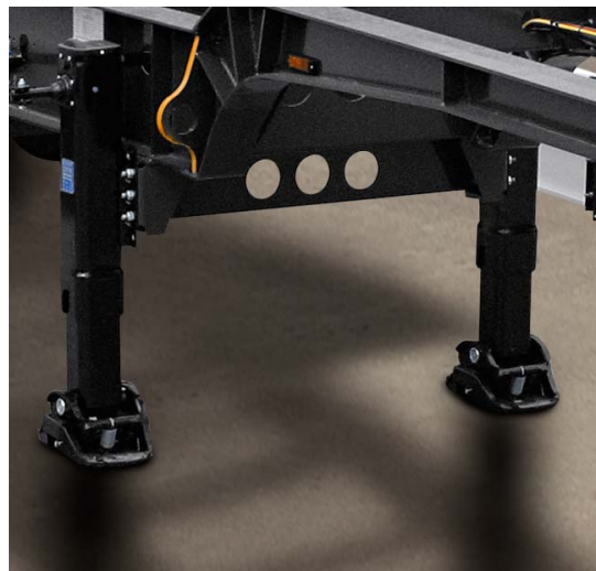
Stable for robust manoeuvring: Landing gear with two-stage gearbox
