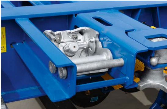
KLAPP LOCK locking mechanism: In lowered position (top) and folded out as the rear lock for the front container for 2 x 20' loading.
