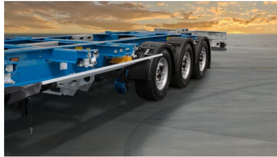
Greater ground clearance: The side guard can be folded up.
