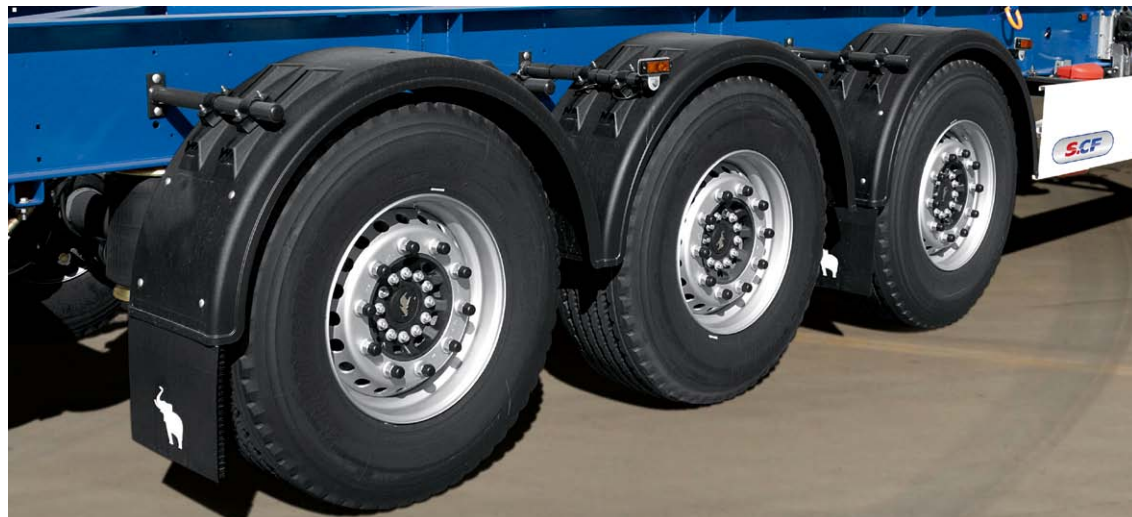
Reduce spray: Anti-spray mud flaps and shell mudguards.
