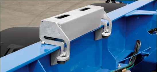
Option: Three pairs of folding container supports for 40'/45' containers without tunnel.
