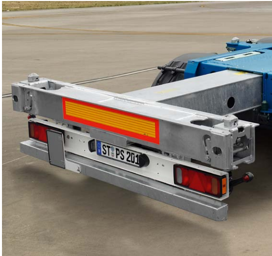
At the press of a button: The rear extension is pneumatically set to the specified container size and locked in place.
