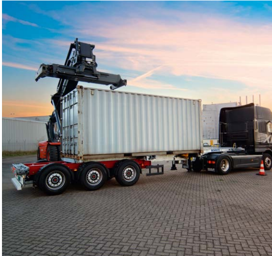
Extending the container frame to the 5,850 mm wheelbase enables 20' containers to be positioned flush with the ramp for unloading.
