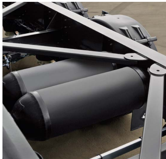
Steel/metal compressed air tank.
