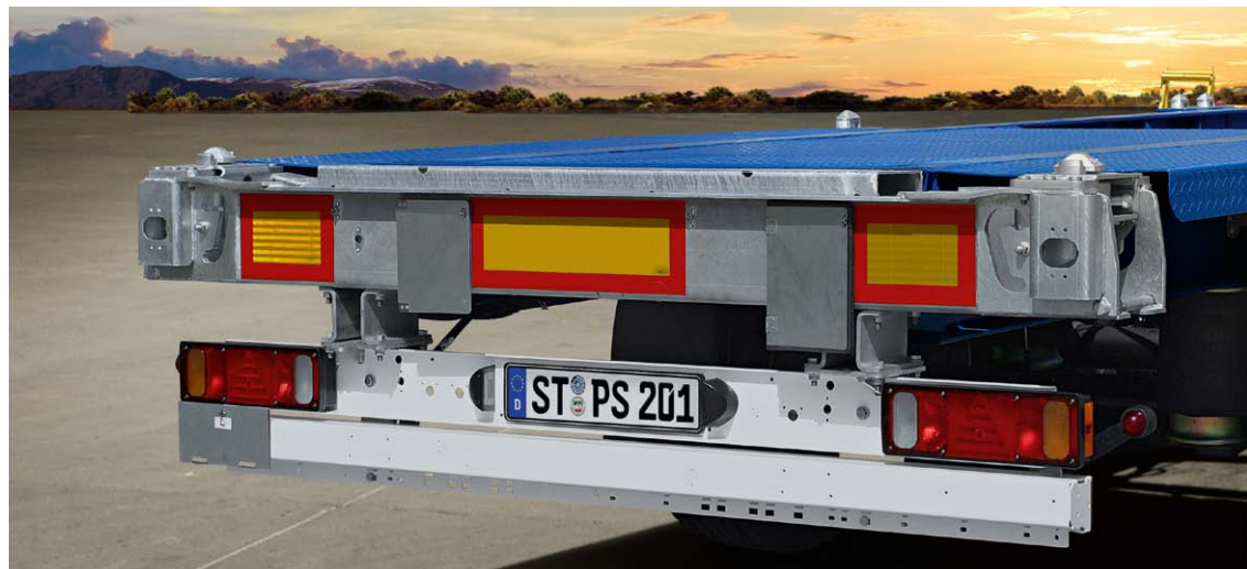
Warning sign, ECE 70/01 Type III for semitrailer chassis on the rear beam / folded warning signs.
