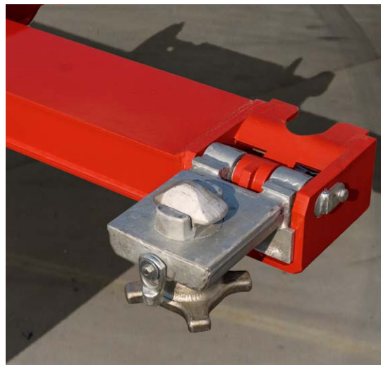
Folding locks on the rigid front beam for TWIST LOCK.
